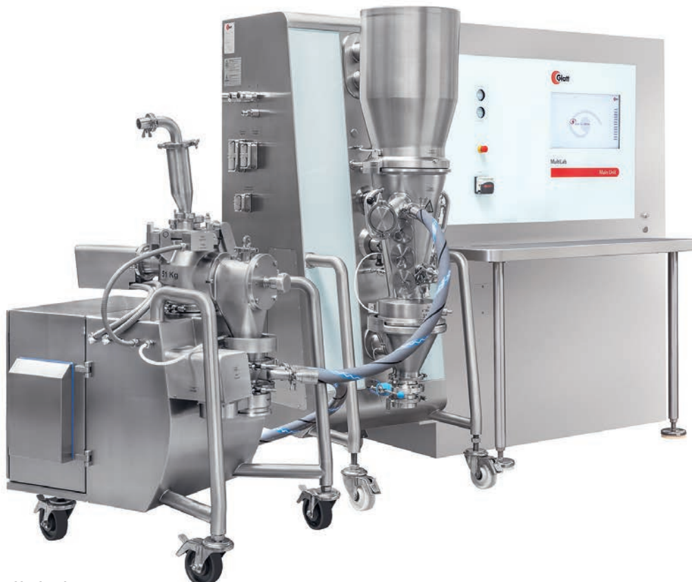
MultiLab with fluidized bed and VG
