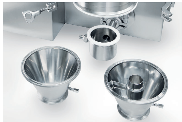
Granulation and Bottom Spray insert
