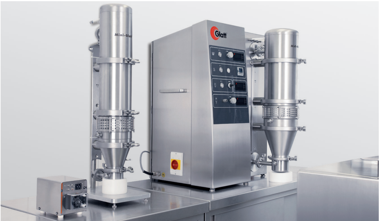
Midi-Glatt with Mini-Glatt interchangeable machine tower
