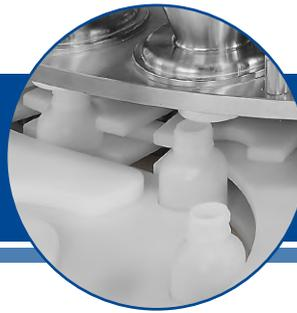
The CVC 6088-2R24 Automatic Rotary Powder Filling Machine is designed to fill powder products into containers provided to its infeed conveyor and transported through its rotary continuous motion mechanism. The Powder dosing uses servo motor driven auger dosing system for accuracy volume.
