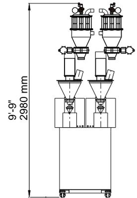
The dimensions shown are for standard machine with optional infeed and outfeed conveyor. Optional conveyor for bottle transportation is available upon request. This machine with an optional conveyor can run independently or be integrated into an automated packaging line. All CVC equipment is covered by a one-year parts warranty. Full Warranty details are included in our equipment proposals or can be found on our website.
