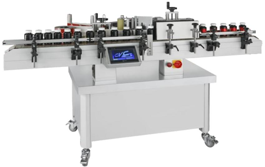
All CVC labelers include our patented Self Set™ software which utilizes a high frequency encoder for extremely easy setup and wrinkle free labeling at the touch of a button.
