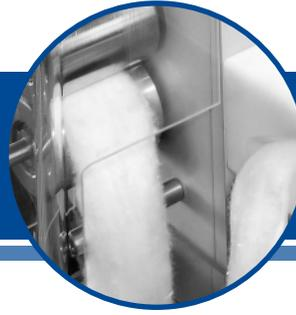
The CVC 1117 Series of Cotton Inserter is designed to insert polyester, rayon, or cotton coil into
