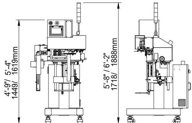
The dimensions shown are for standard machine. The conveyor can be extended: the length may vary based on selected options. This machine can run independently or be integrated into an automated packaging line. All CVC equipment is covered by a one-year parts warranty. Full Warranty details are included in our equipment proposals or can be found on our website.
